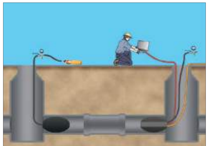
The test of leakage with air according DIN EN 1610
